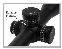
full revolutions of adjustment. The first revolution or 100 clicks are indicated by white scale on the knob. On the second revolution (101 to 195), a small elevation Rotation Indicator pops out at the base of the turret to remind the shooter to use the second scale indicated by grey numbers on the dial.
